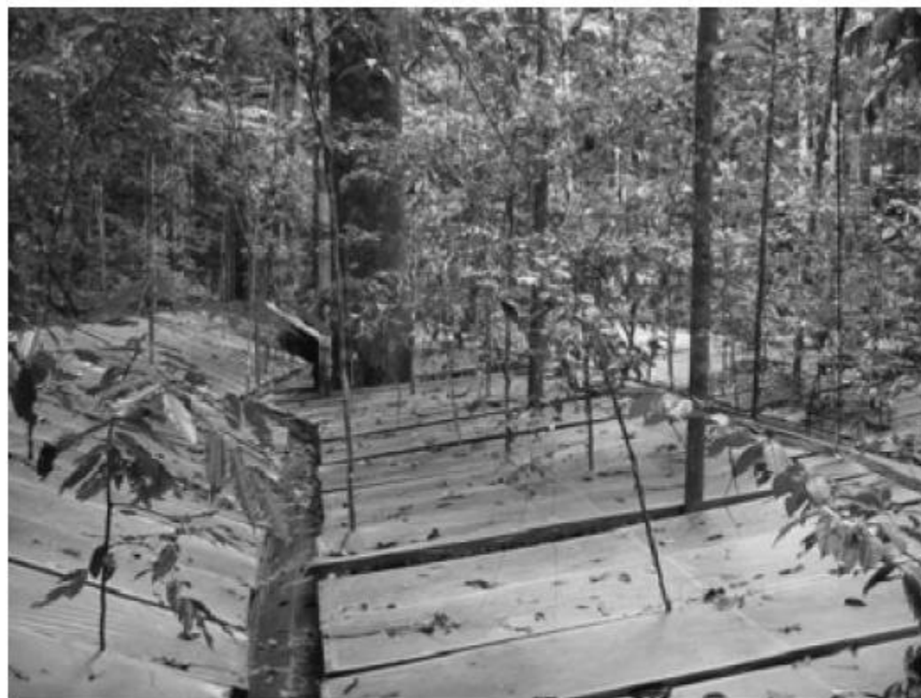
Fig. 1 Throughfall exclusion installation at Caxiuanã forest. One hectare ( 100\text{ m} \times 100\text{ m} ) of plastic panels draining into aqueducts intercepts incoming rain and drains it away from the soil, causing an artificial drought. The panels cover \sim 80\% of the ground area and were in place throughout the whole duration of the experiment, with the exception of the 4–21 November 2002, when they were removed.
